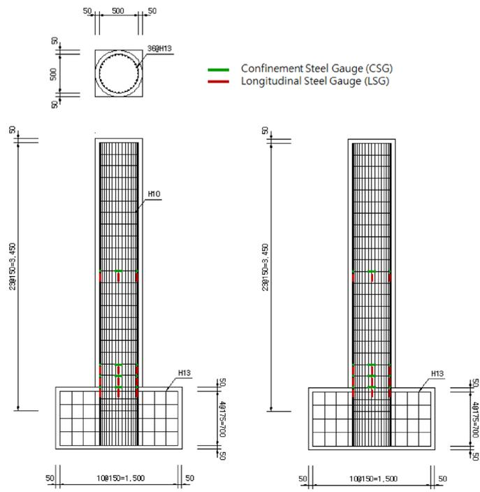
(a) Circular cross-sectional RC column specimen
