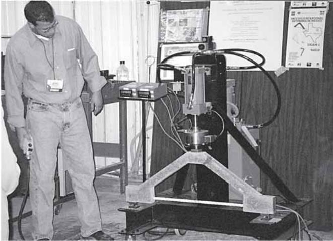
Student competitions, a regular event at conventions, have featured the building and testing of a wide variety of concrete projects: cubes, beams, bowling balls, and egg-protection devices. Pictured is the testing of a fiber-reinforced polymer concrete frame in a 2001 competition.
