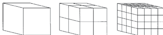
Fig. 3.1.4a—Effect of particle size on aggregate surface area: (a) one 25.0 mm (1 in.) cube of aggregate (surface area = 6 \times 25.0 \times 25.0 = 3750 \text{ mm}^2 [6 in. 2 ]); (b) eight 12.5 mm (1/2 in.) cubes of aggregate (surface area = 6 \times 12.5 \times 12.5 \times 8 = 7500 \text{ mm}^2 [12 in. 2 ]); and (c) sixty-four 6.25 mm (1/4 in.) cubes of aggregate (surface area = 6 \times 6.25 \times 6.25 \times 64 = 15,000 \text{ mm}^2 [24 in. 2 ]).
