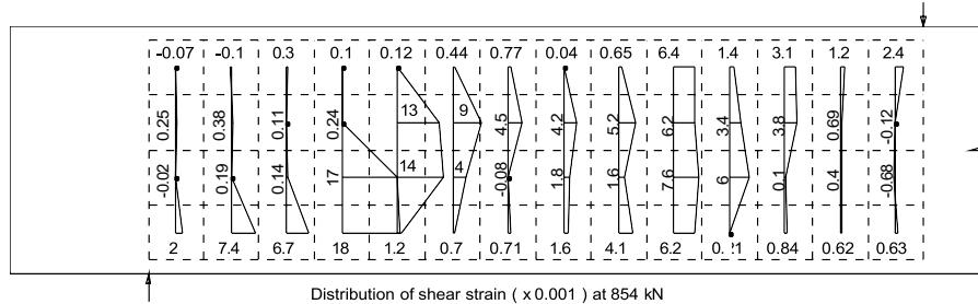
d) Distribution of shear strains at peak load
