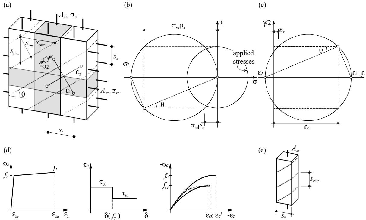
Fig. 2—Cracked membrane in pure shear: (a) stresses in concrete and steel; (b) Mohr's circle of stresses and (c) strains; (d) constitutive laws for steel, bond shear stress-slip and concrete; and (e) equivalent tension chord with stirrup reinforcement.
