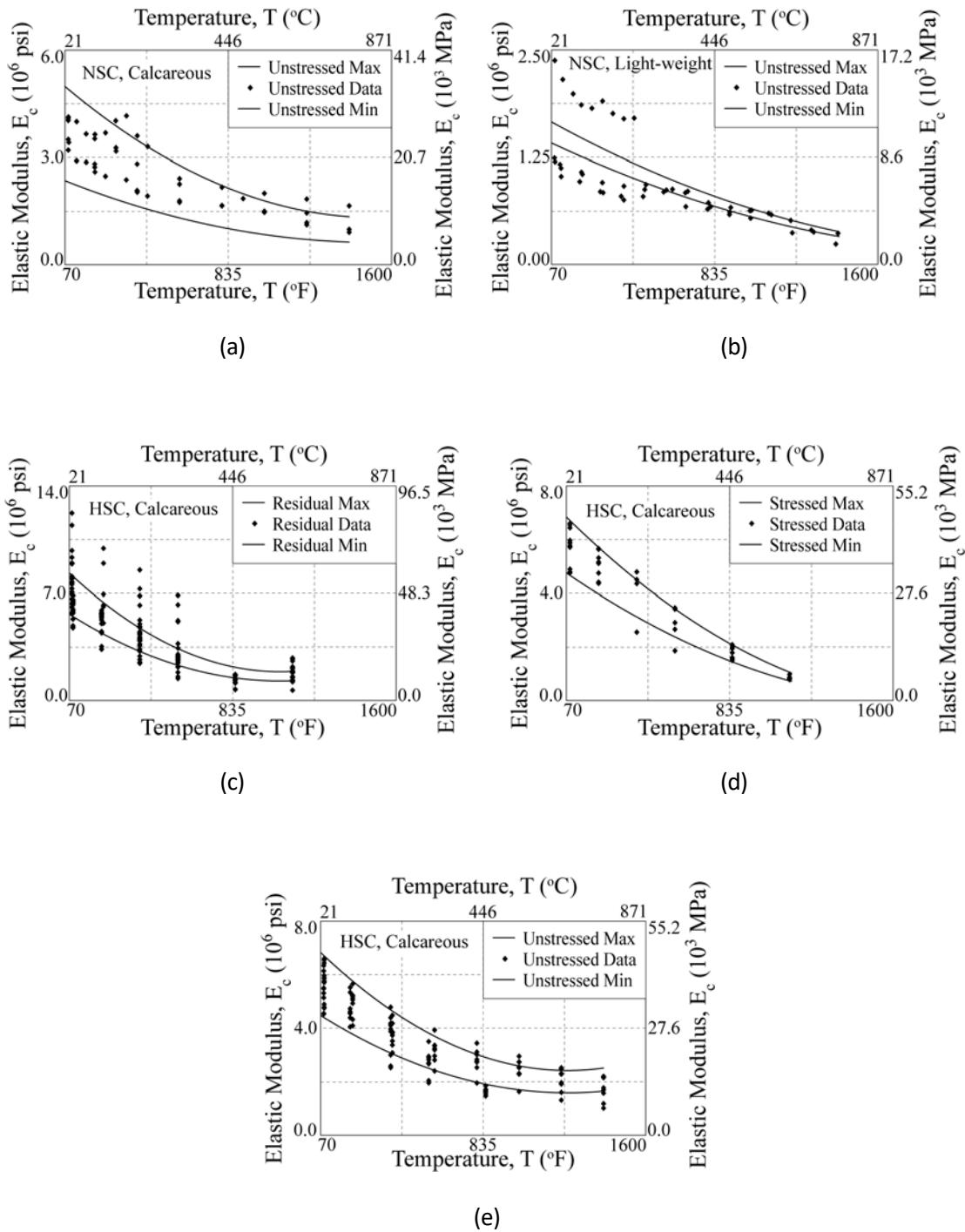
Fig. 1—Proposed  $E_c$  model prediction bands: (a) NSC, calcareous, unstressed; (b) NSC, lightweight, unstressed; (c) HSC, calcareous, residual; (d) HSC, calcareous, stressed; and (e) HSC, calcareous, unstressed.
