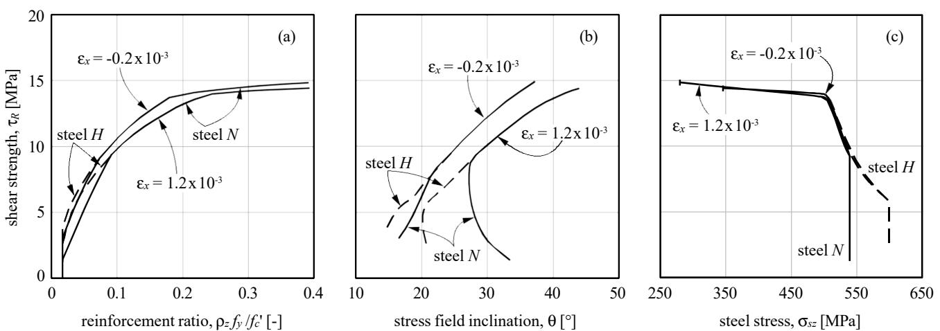
Fig. 3—Results for membrane elements with  $f'_c = 50$  MPa and  $f_y = 500$  MPa, longitudinal strains
