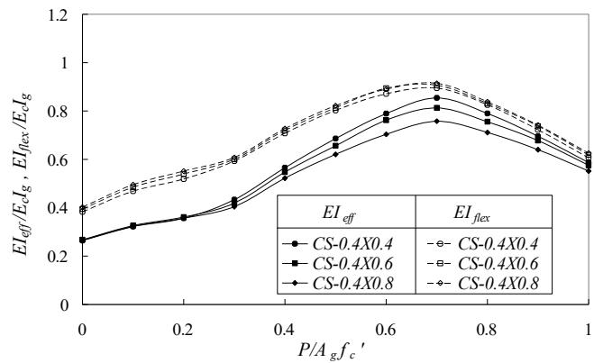
*Fig. 1—Variation of flexural and effective stiffness ratios with axial load ratio for different depths of member. (Note: CS denotes cross section size in m; 1 m = 39.37 in.)*
