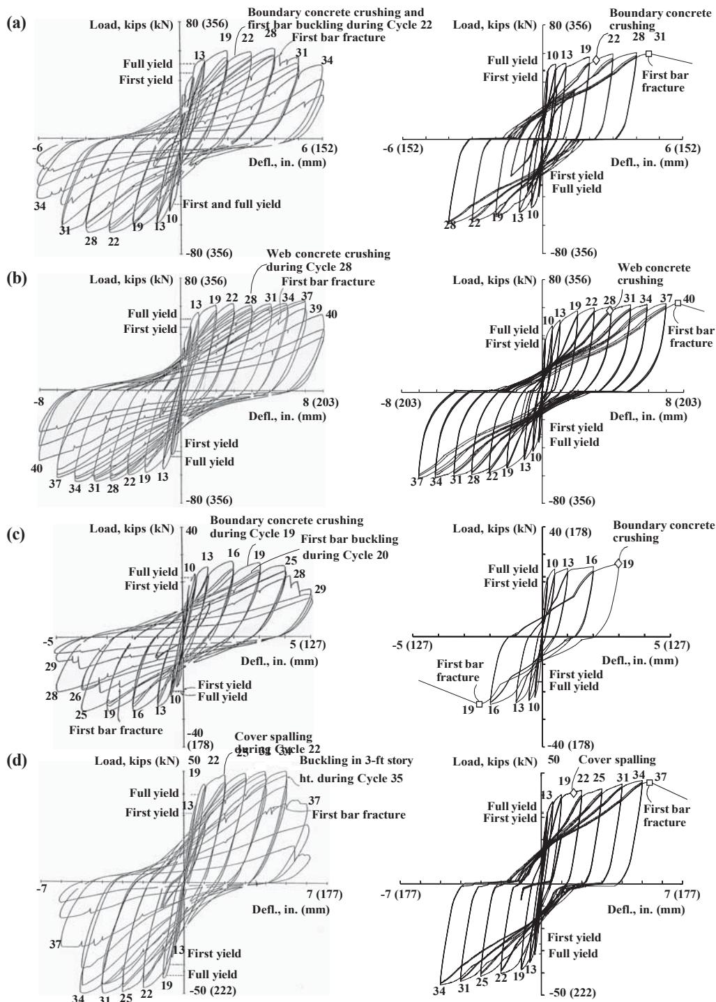
Fig. 2—Estimated (right) and measured (left, from Oesterle et al. 1976, 1979) lateral load versus deflection behaviors: (a) Wall B1; (b) Wall B3; (c) Wall R1; and (d) Wall R2.
