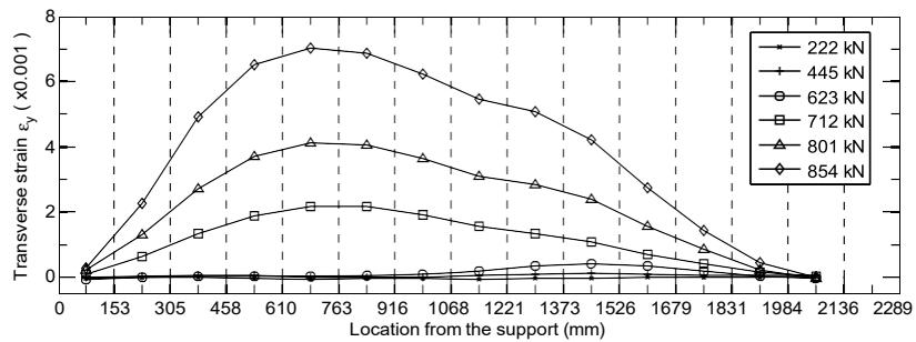
b) Vertical strains at various loads, averaged over beam depth
