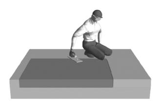
Fig. 10—After floating, trowel or broom the surface.
