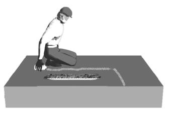
*Fig.* 2—*Mark the perimeter of the repair area using simple geometric shapes and minimizing re-entrant corners.*
