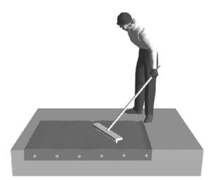
Fig. 9—Strike off, then float the repaired surface.
