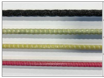
BasaFlex<sup>TM</sup>, BFRP Rebar, Basanite Industries https://www.basaniteindustries.com/products.html
