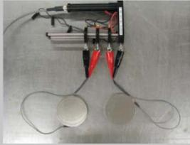
Wires from plates are attached to Wenner probe tips.
