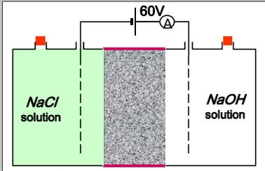
Voltage is applied and current passing through concrete is measured and integrated over 6 hours to get charge passed in Coulombs
