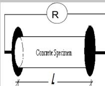
And calculate resistivity accounting for Area and Length of sample
