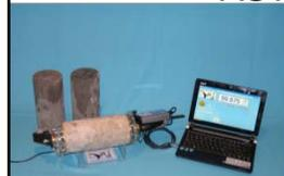
The resistivity Test take less than 1 minute and the same sample can then be used for strength testing
