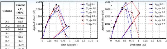
Increasing  $f'_c$  seems to decrease the drift at the peak of  $V_c$ , thus reducing the corresponding stress in the transverse reinforcement.
