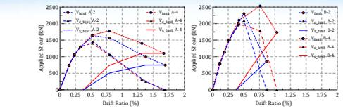
Decreasing vertical spacing of transverse reinforcement seems not affecting the degradation pattern of  $V_c$ . However, due to the increase of  $V_s$  for a given drift,  $V_n$  is still able to increase after the peak of  $V_c$ , thus increasing  $V_n$  and the stress in transverse reinforcement at the peak of  $V_n$ .
