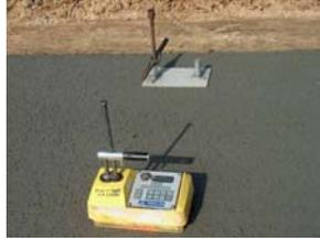
Nuclear Gauge | ASTM C1040
