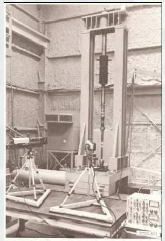
Figure 2.29 Instrumented specimon in place ready for testing.
