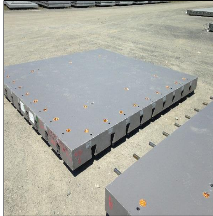
Finished Slabs (stainless steel dowels and rebar)
