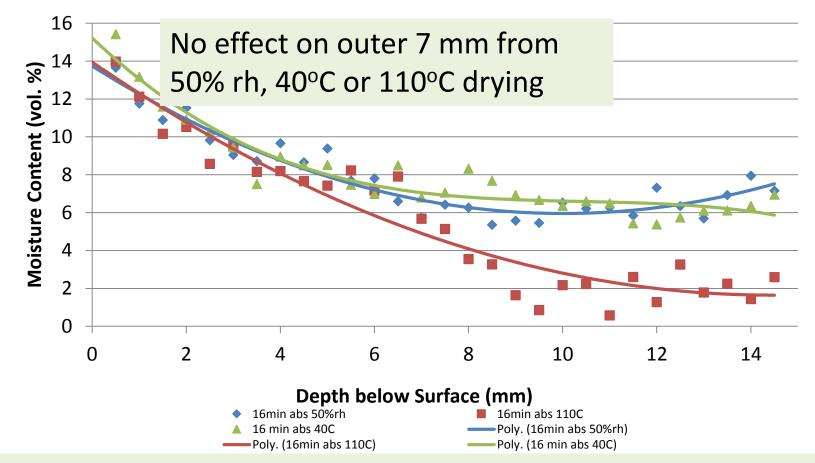
We know 110°C drying damages concrete but does not appear to affect absorption profile relative to 40°C drying, except for different starting moisture content
