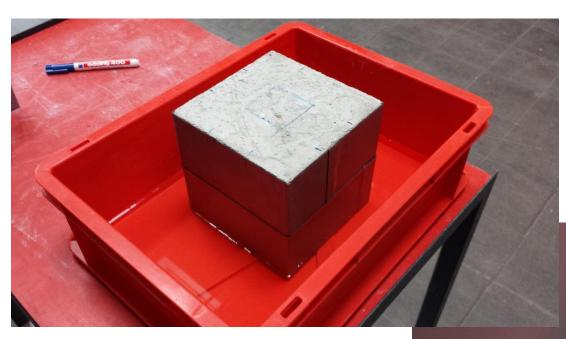
One profile was measured for each absorption time in the centre of the exposed cube surface
