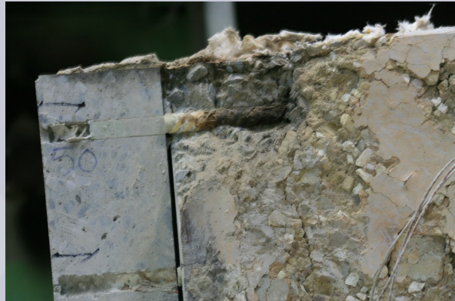
Post-fire condition of FRP bar in cool zone
