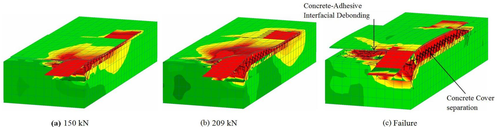
**Figure** – FRP debonding failure progression(FEM Model) depicting exaggerated deformations;
