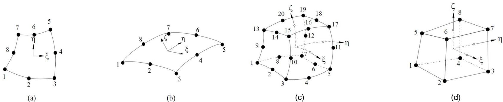
Figure - (a) Typical eight-node quadrilateral isoparametric plane stress element; (b) Typical eight-node quadrilateral isoparametric curved shell element; (c) Typical twenty-node isoparametric solid brick element and (d) Typical eight-node isoparametric solid brick element
