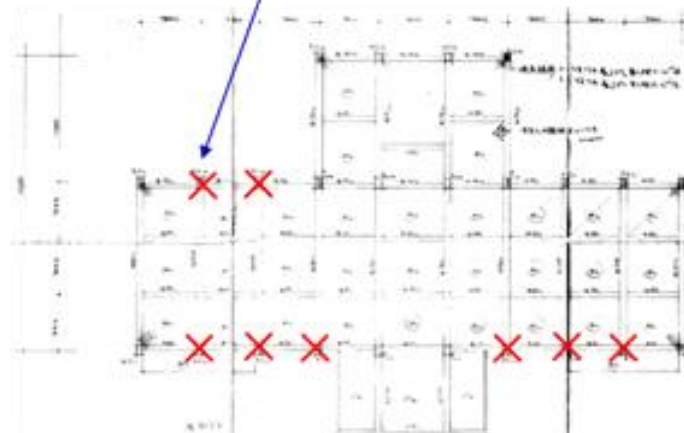
Observed Column Damage during Meinong Earthquake
