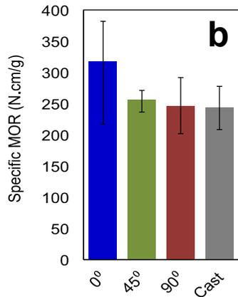
➤ No significant differences between strength of cast and printed specimens
