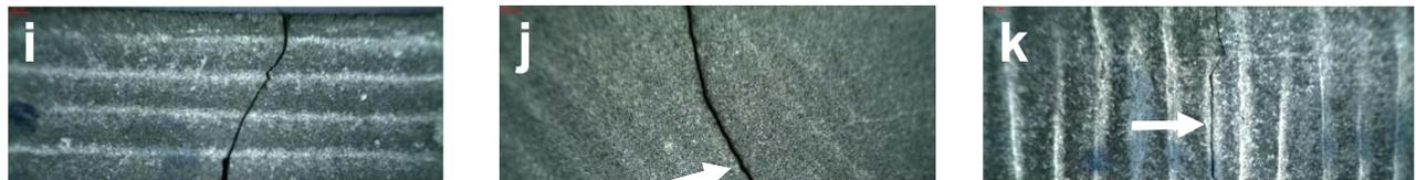
**Weak interfaces can be utilized to control the crack path and to improve fracture properties**
