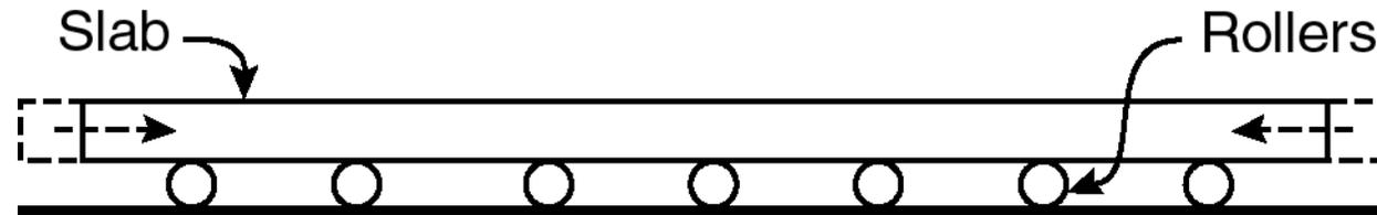
Shrinkage + freedom to move = no cracks
