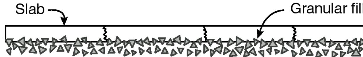
Shrinkage + subbase restraint = cracks
