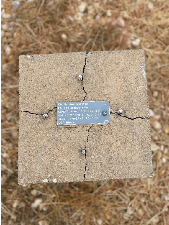
Type: Cement D Type III (700 lb) Max Temp: 178
