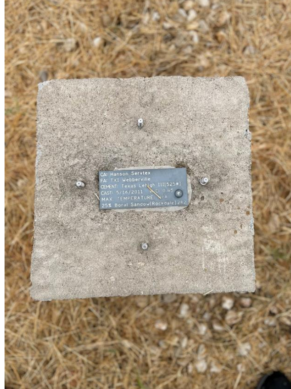
Cement D – Type III (525) 25% Class F Fly Ash
