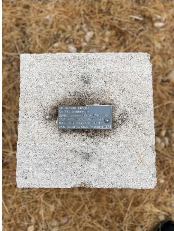
Type: Cement M – Type White (700) 25% Class F Fly Ash Max Temp: 194
