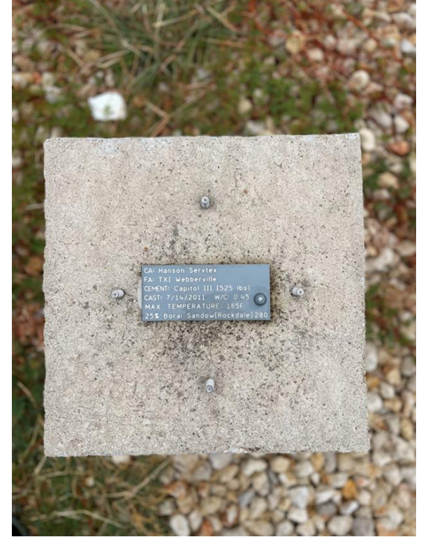
Type: Cement C – Type III (525lb) 25% Class F Fly Ash Max Temp: 185
