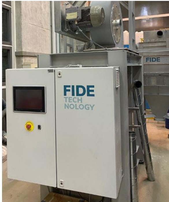
FIDE LC Mill Prototype at EPFL with a capacity of 150 kg per hour
