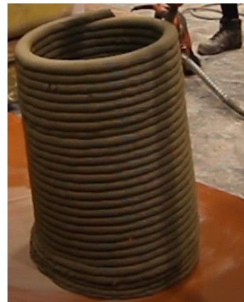
Plastic collapse Concre3DLab Ghent
