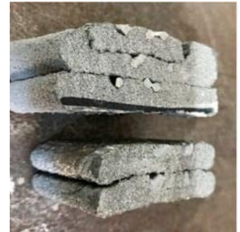
Weak bonds and cold joints
