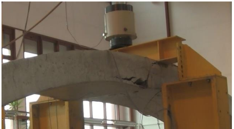
Crack initiation in L/2
