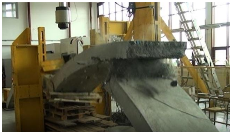
Element during final failure
