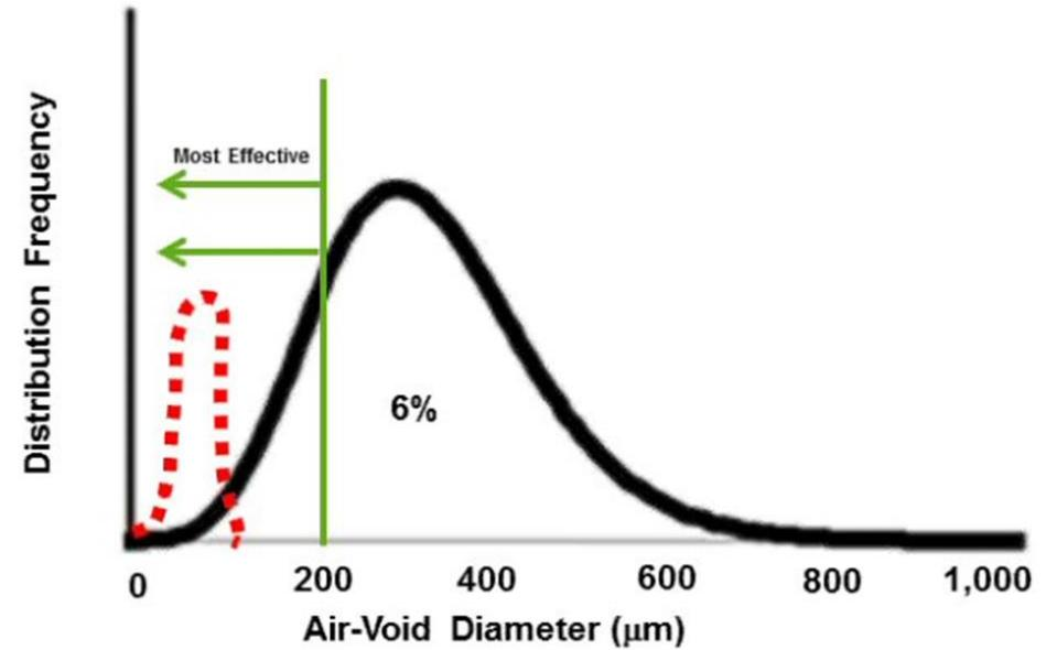
A 1%-dose (by volume) of 40- $\mu\text{m}$  spheres produces 22,000,000 spheres per cubic foot of concrete
