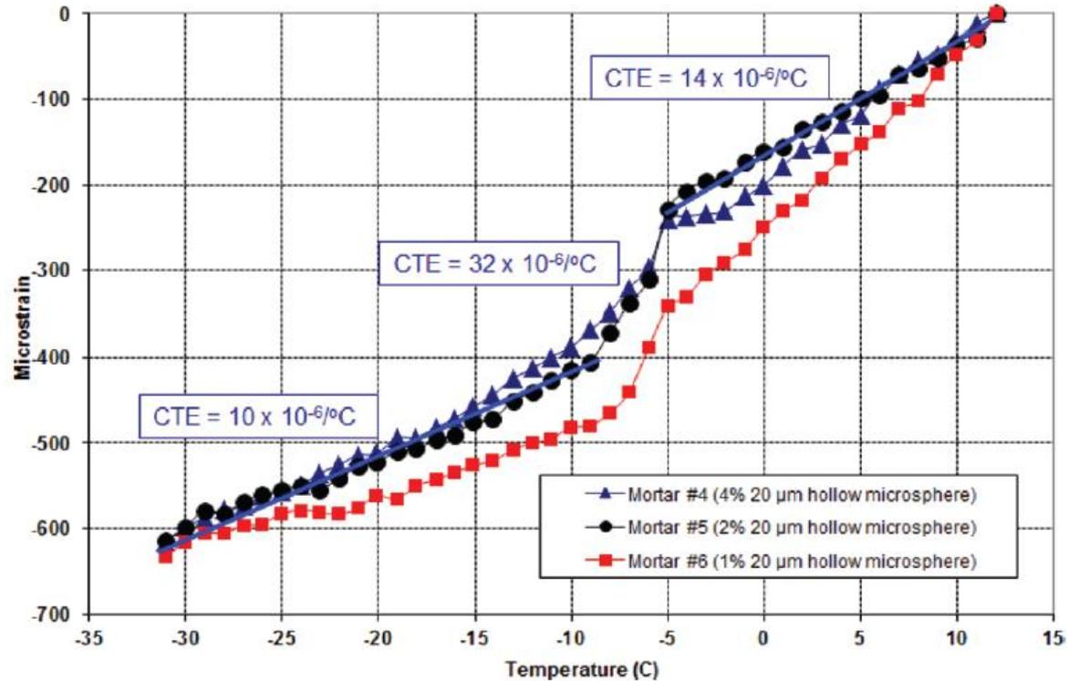
Microstrain as function of temperature during freezing for mortar containing 1, 2, or 4% by volume of 20 µm diameter hollow (compressible) microsphere during first cycle of testing.
