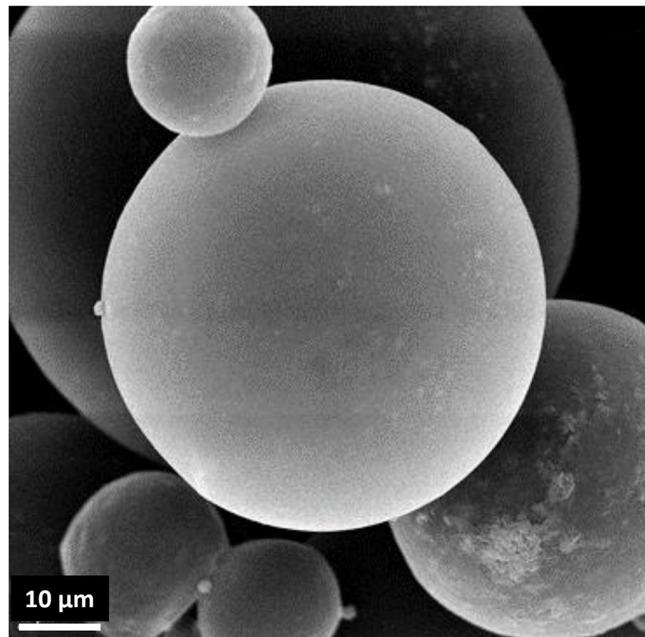
Polymeric microspheres with nominal diameter of 40 μm
