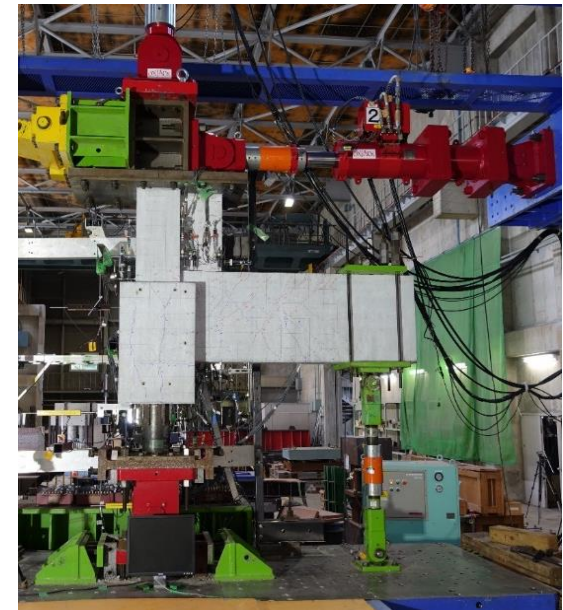
Column-beam-pile connection (smaller scale)
