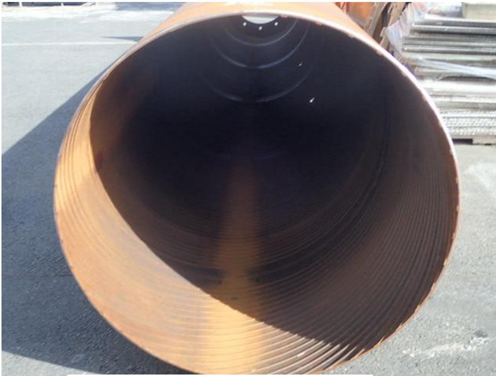
Internal ribs of steel tube ( \Phi = 1200\text{mm} )
