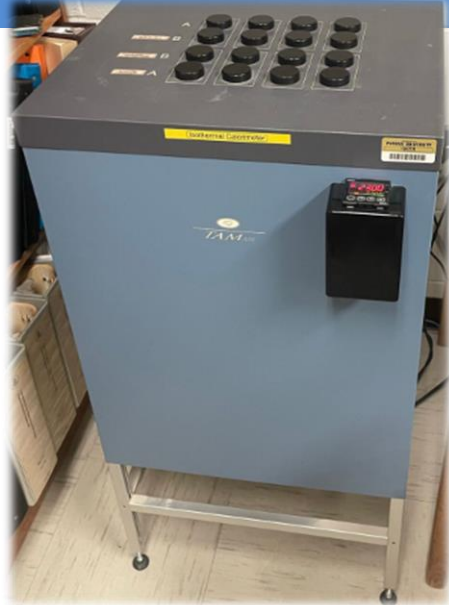
Isothermal Calorimetry ASTM C1679
