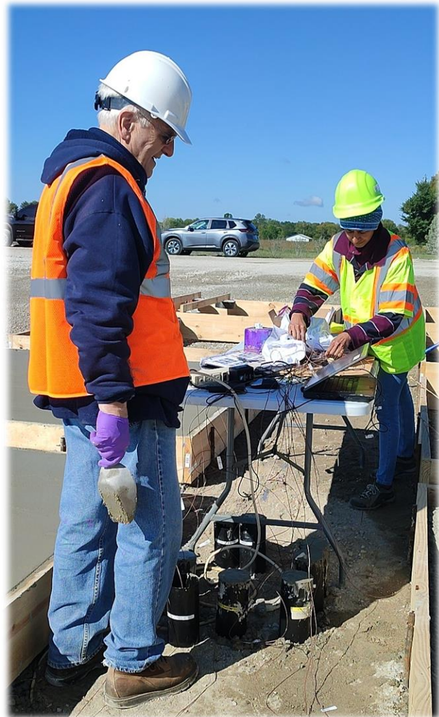
Thermocouples installed in slabs and cylinders connected to Data logger
