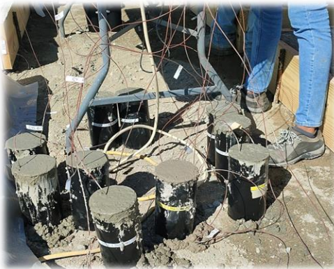
Thermocouples installed in slabs and cylinders connected to Data logger
