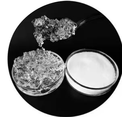
Superabsorbent polymer Polyacrylamide-based particles dry diameter < 300 \mu m
