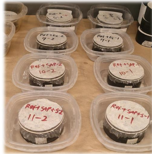
Rate of Water Absorption ASTM C1585
