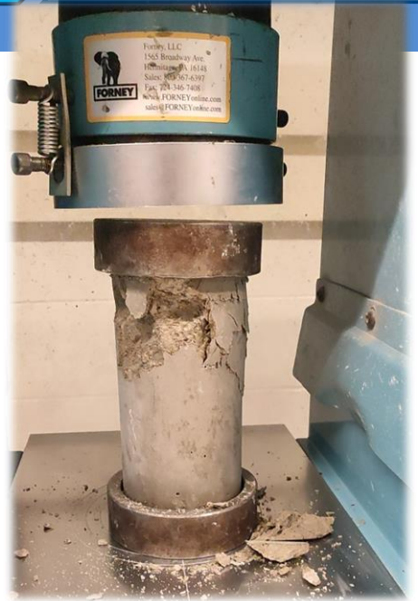
Compressive Strength Testing ASTM C39
