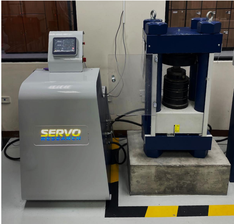
Compressive strength setup with 3000kN capacity load and displacement controlled.
