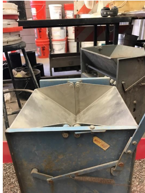
Mechanical Splitter used to obtain uniform gradation of particles
