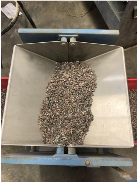
Mechanical Splitter used to obtain uniform gradation of particles
