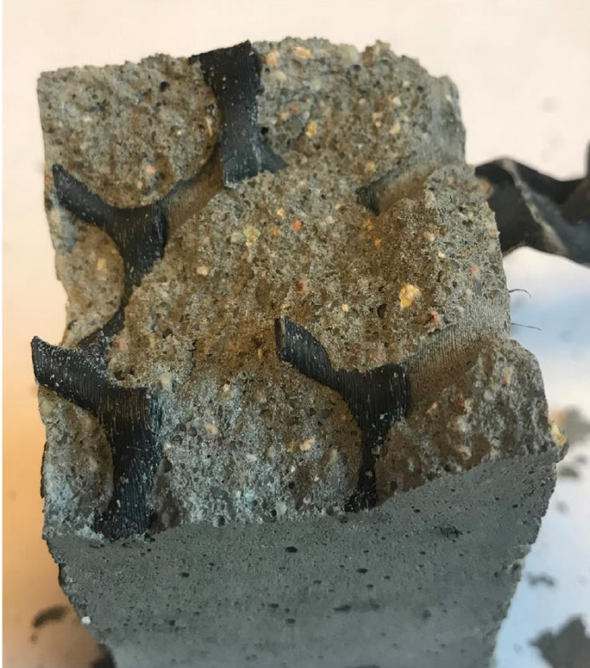
Plastic gyroid reinforced concrete beam, Skoratko 2022
