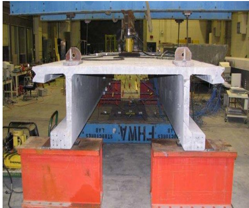
Pi section bridge girder
