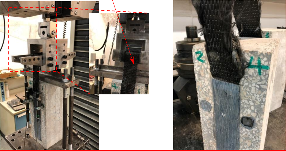
U-shape dry fibers over rollers
