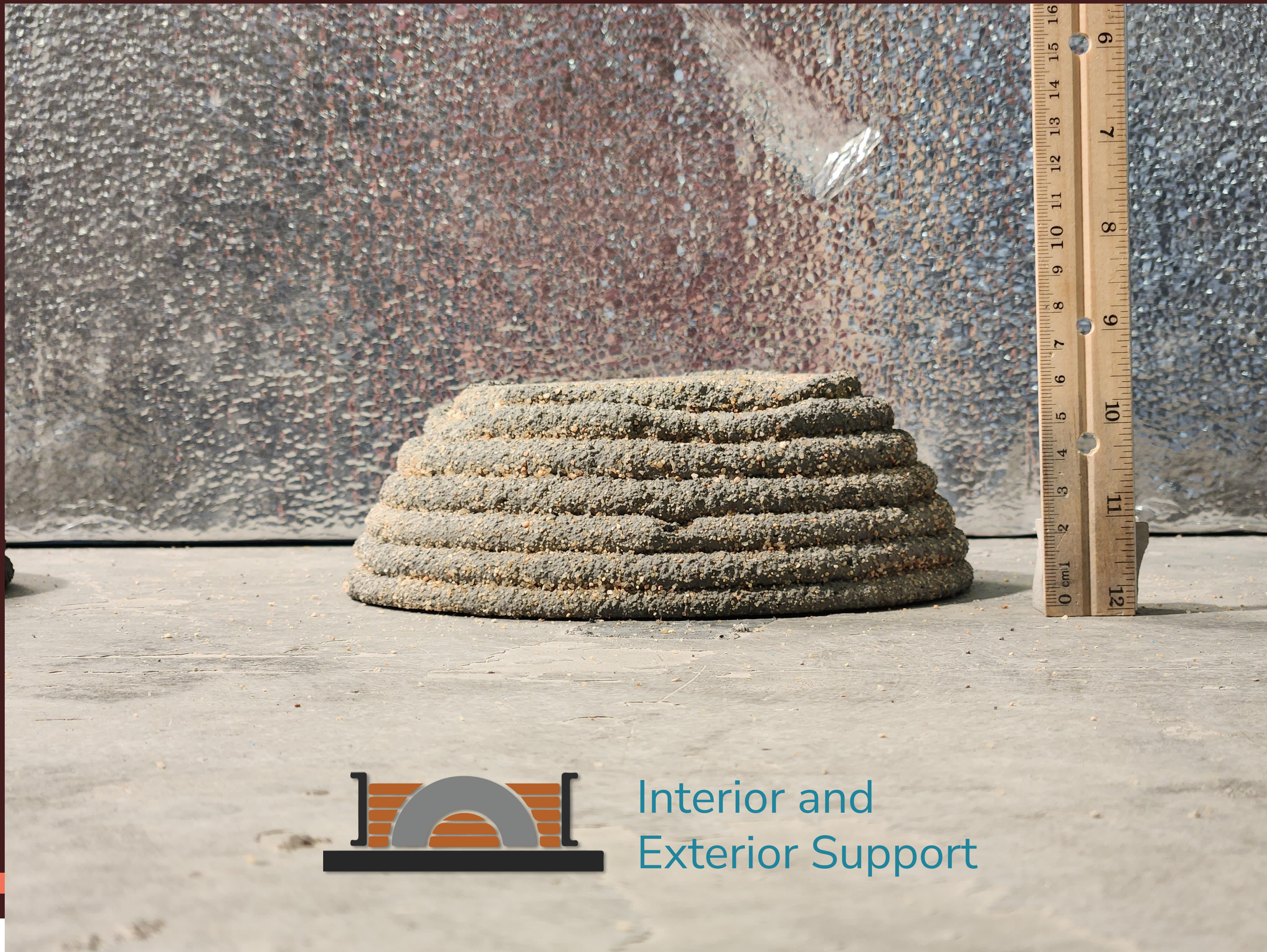
Print 4: W/C 0.38 With Weight Applied
