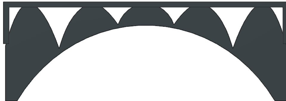
Optimized Compression-Only Design (Arch Structure)
