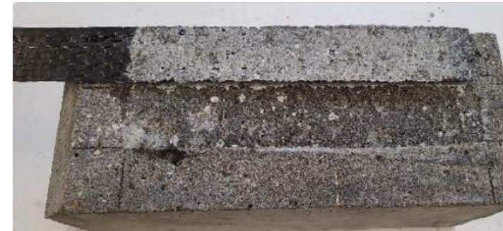
Adhesive failure in the adhesive/concrete interface (300 cycles)
