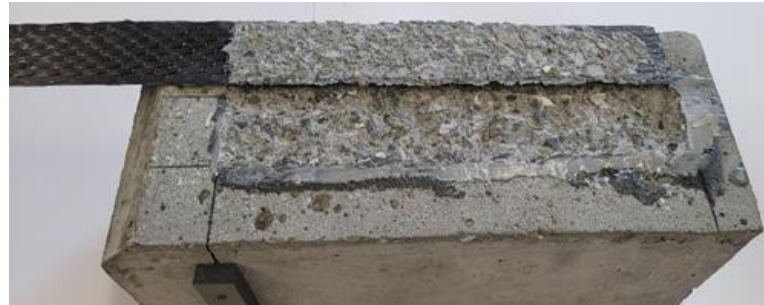
Cohesive failure in concrete with 2mm (Control samples)
