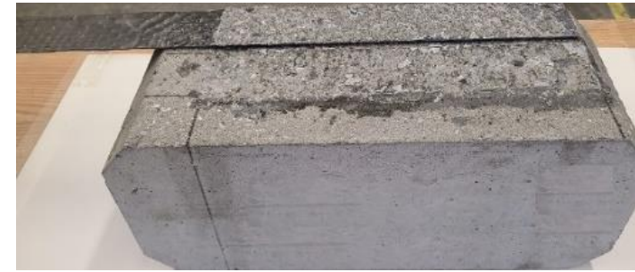
Cohesive failure in concrete with 1 mm (100 cycles)
