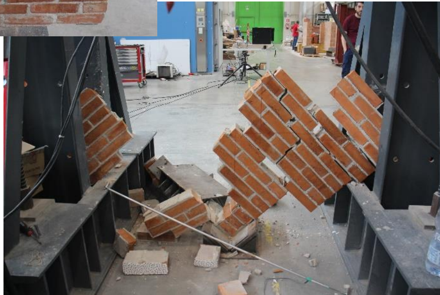
Diagonal cracking (very fragile)
