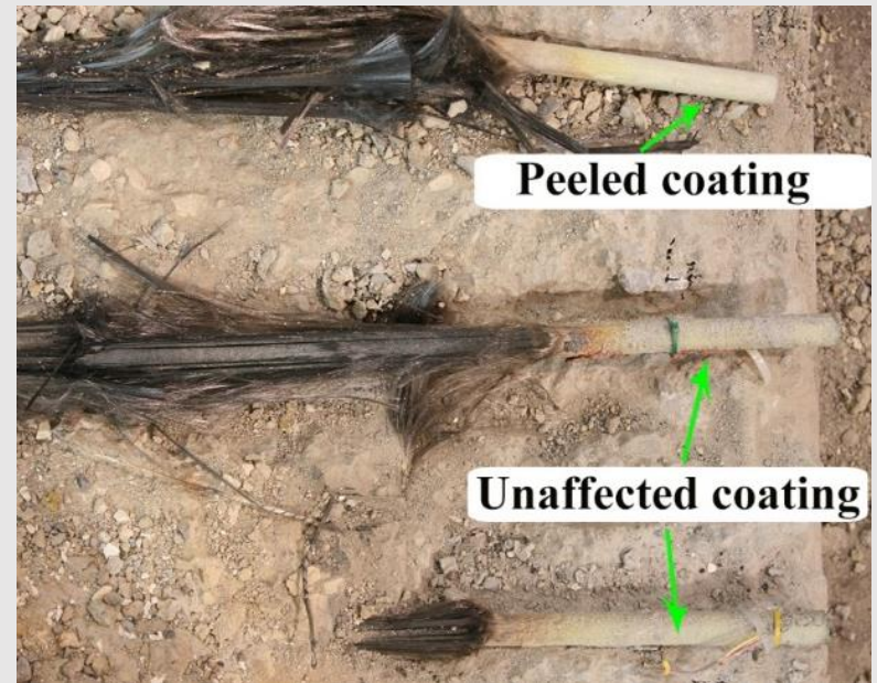
Condition of bars in the exposed and unexposed zones
