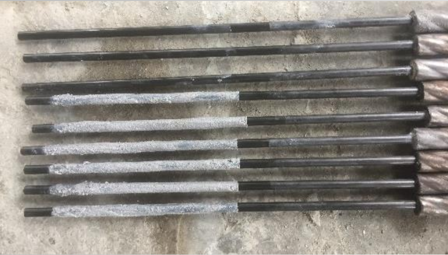
CFRP bars: smooth bar and coated with Sikadur-30 (average of 1 mm thickness)
