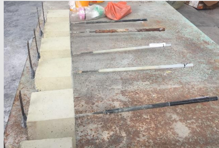
CFRP bars: deep embedment
