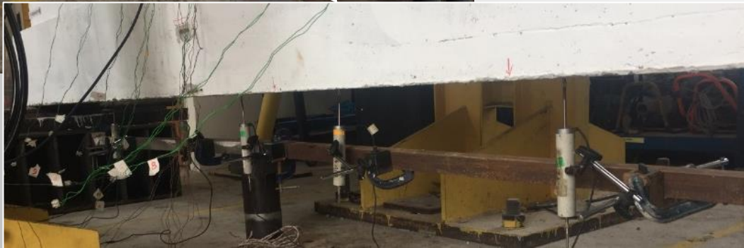
Four points flexural test set up in the laboratory
