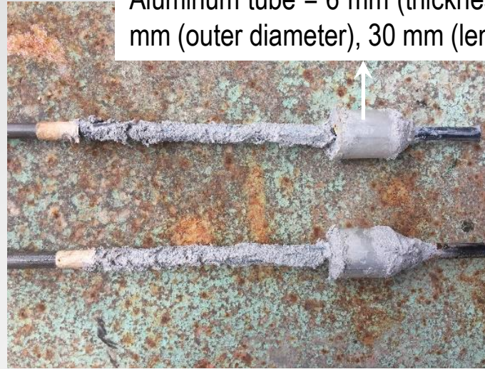
CFRP bars: coated with Sikadur-30 (average of 1 mm thickness) and additional anchorage
