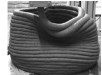
3D-printed concrete structure failure due to insufficient buildability
