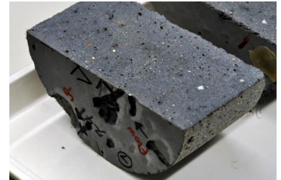
Cut plane parallel to crack
