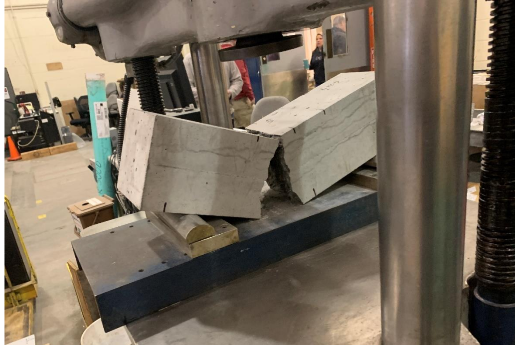
Traditional brittle behavior of concrete
