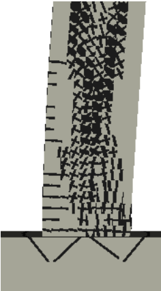
Simulated deformed shape and crack patterns
