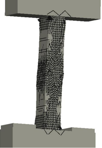
Simulated deformed shape and crack patterns
