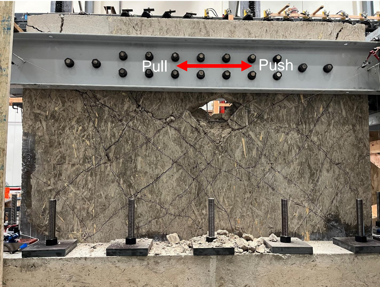
6" wall with 0.14% shear reinforcement ratio (Type 1)
