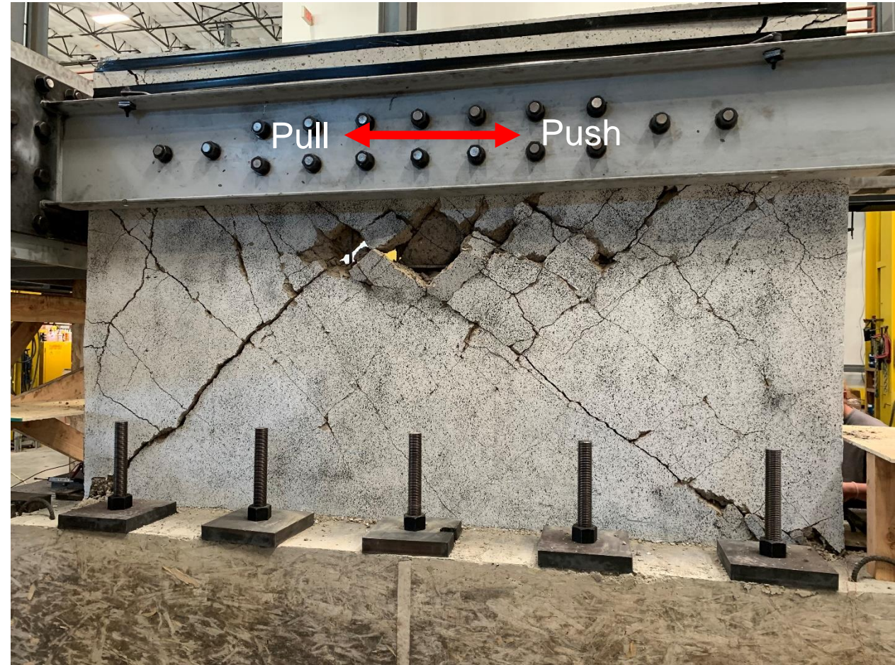
6" wall with 0.26% shear reinforcement ratio (Type 2)
