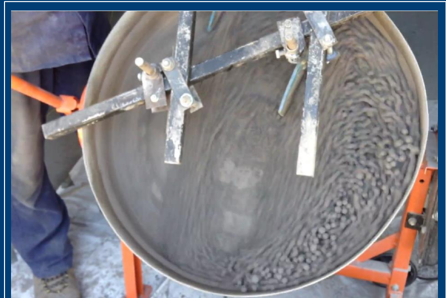
Figure 3 shows formation of Pellets using Pelletizing Disc
