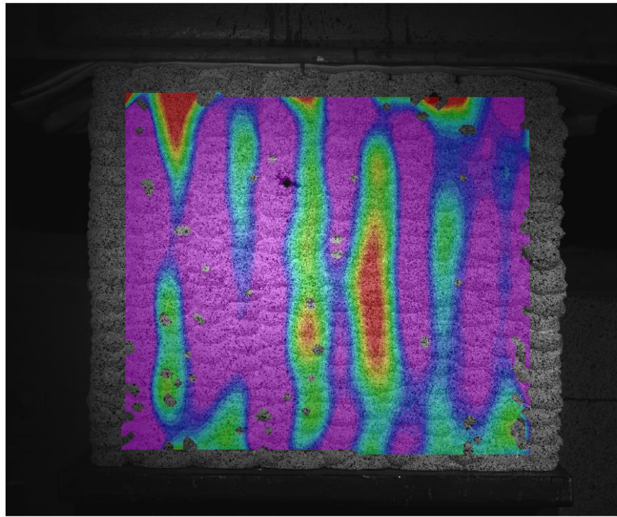
Strain along direction-3 from DIC analysis (near 50% loading of crack initiation load).
