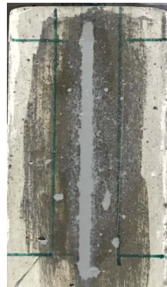
Application of epoxy adhesive
