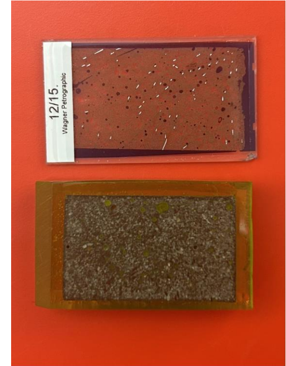
Standard micron thin sections using high pressured fluorescent epoxy impregnation.
