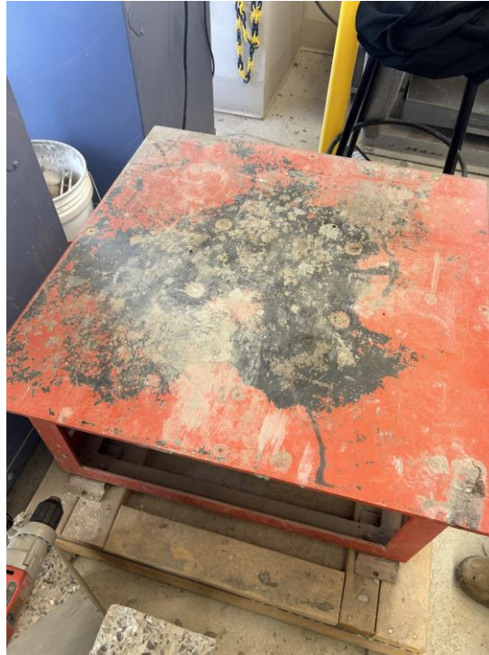
Vibrating table used for consolidating samples.
