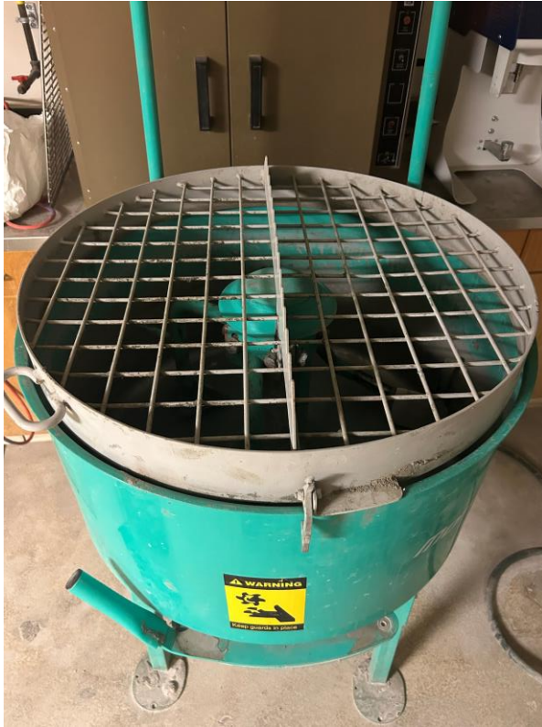
Vertical high-shear orbital mixer (as opposed to a rotating gravity mixer).
