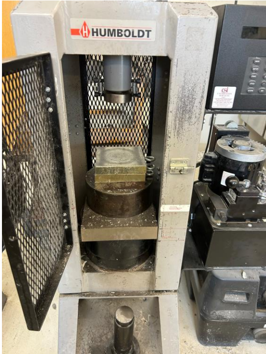
Hydraulic press to test for the compressive strength of samples.
