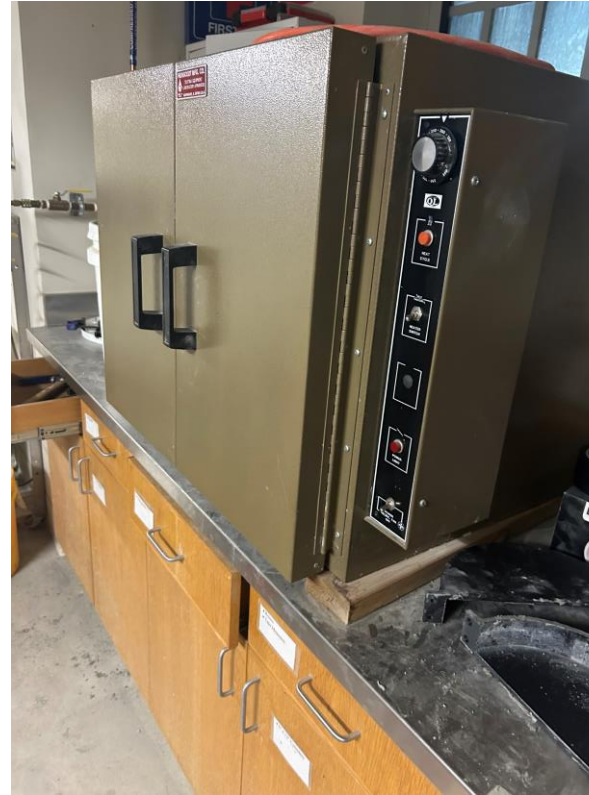
Steam/submergence apparatus made using ovens and bowls/buckets of water.
