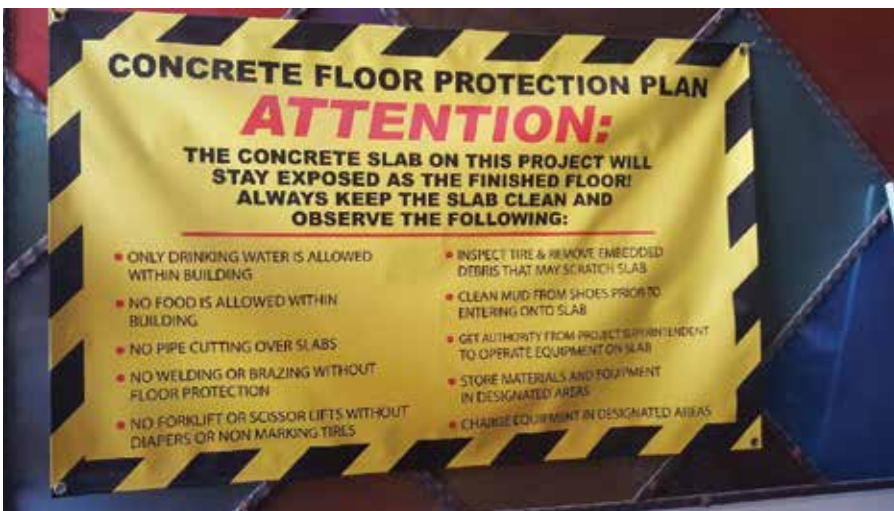
Signage can be an effective part of jobsite implementation
