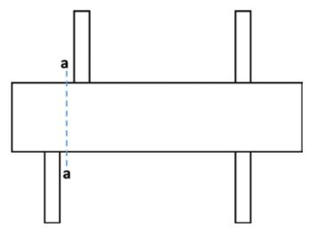
Fig. 6: Transfer girder at an offset in the column grid
