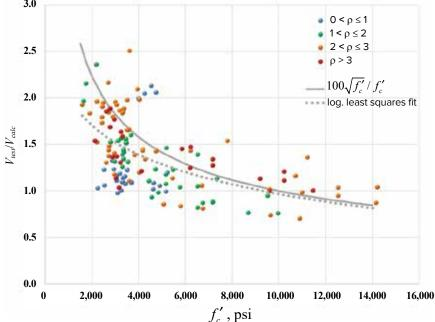
Fig. 3:  $V_{test}/V_{colc}$  versus  $f'_{c}$  (Note:  $V_{colc}$  in accordance with the strut-and-tie method in ACI 318-14;  $\rho$  = longitudinal reinforcement ratio, %)
