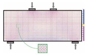
Fig. 2: Example of stress flow in a deep beam. Blue lines in the inset indicate tension orientation
