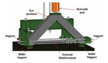
Fig. 4: Schematic of test setup and specimen with supports (truss-like specimen shown)
