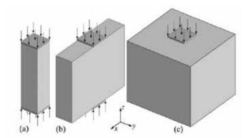
Fig. 1: Illustrations of: (a) rectangular prismatic strut; (b) 2-D rectangular bottle-shaped strut; and (c) 3-D rectangular bottleshaped strut (after Laughery and Pujol<sup>4</sup>)
