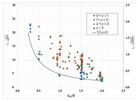
Fig. 7: Shear stress  $v_c$  versus ratio of shear span to effective depth,  $a_v/d$  (Note:  $v_c = V_{test}/bd$ )
