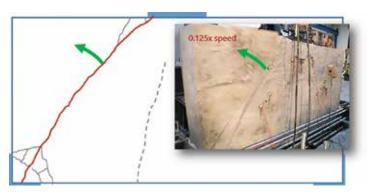
Fig. 5: Failure crack pattern and image of instant of failure for specimen Re-45-Ex
