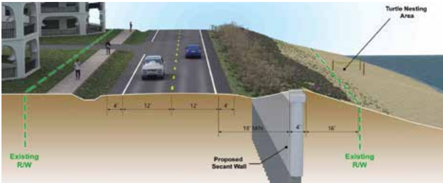
Fig. 2: A schematic rendering of the SR A1A secant-pile seawall/bulkhead project with dune reestablishment and existing right-of-way (r/w) limits
