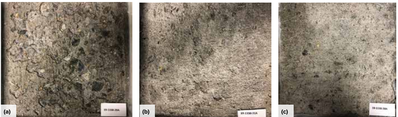
Fig. 6: Surfaces of concrete specimens prepared with w/c = 0.42 after 50 cycles of salt-scaling testing per ASTM C672/C672M: (a) non-air-entrained concrete; (b) air-entrained concrete; and (c) microsphere concrete
