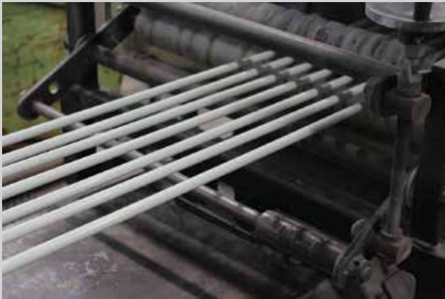
Step 2: The pultrusion process creates glass fiber/vinyl ester composite rods in up to 80 ft (24 m) lengths
