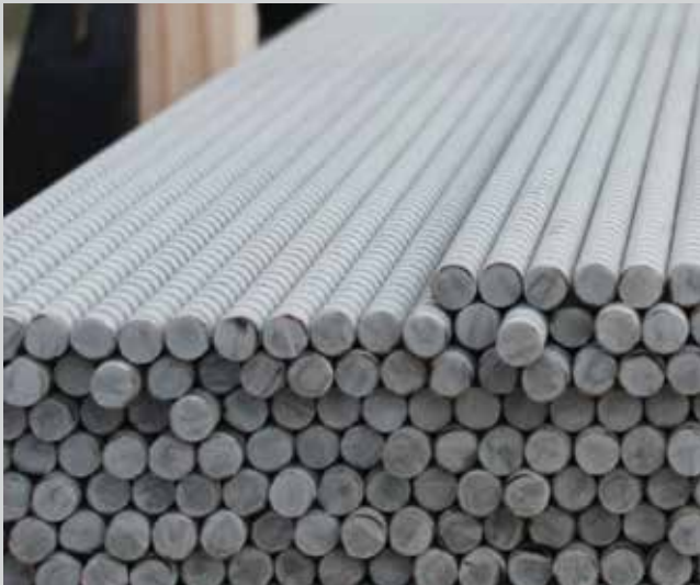
Step 3: A spiral is machined into the rods to assist with adhesion in the concrete
