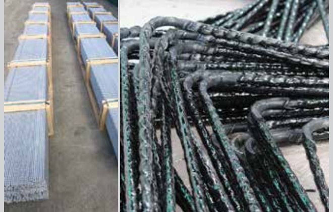
Step 4: Straight and bent GFRP reinforcing bar is shipped to the construction site
