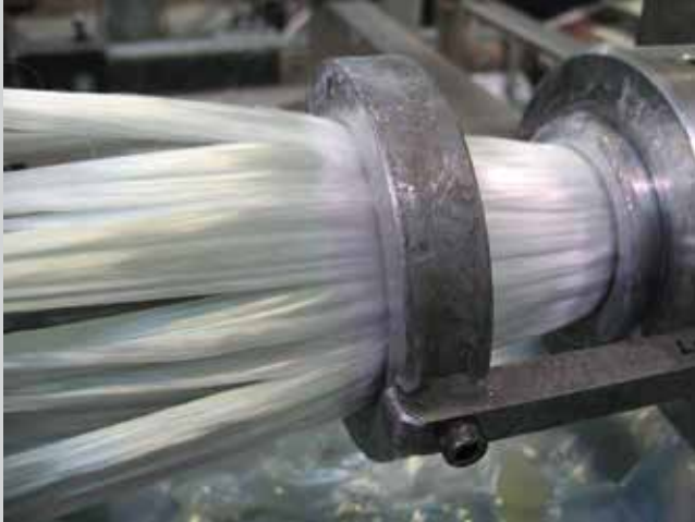
Step 1: Glass fiber is fed into the pultrusion die and injected with resin in a closed-molding process
