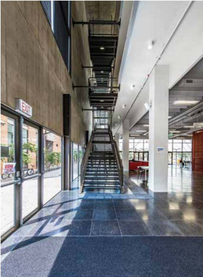
Fig. 2: Staircases and open space between the concrete façade and the inner core allow natural light to enter the building
